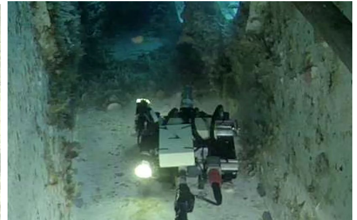
Fairlead internal AFTER Caviblaster cleaning
