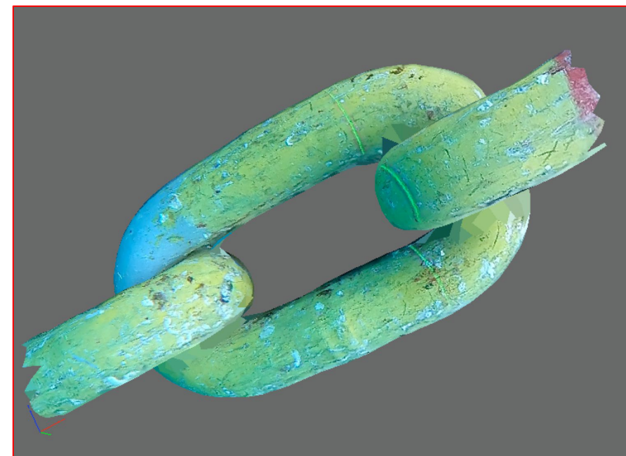
Mooring Chain Measurable 3D Model
